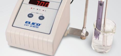
Microcontroller based with Automatic and Manual Temperature Compensation.
